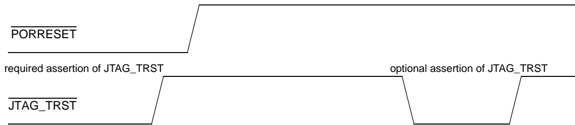
Figure 53. \overline{\text{PORRESET}} vs. \overline{\text{JTAG\_TRST}}
